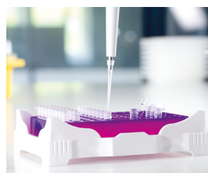
0.5 – 20 µl pipette tips in PCR tubes
