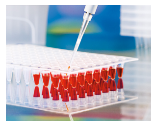
0.5 – 10 µl filter tips in PCR plate
